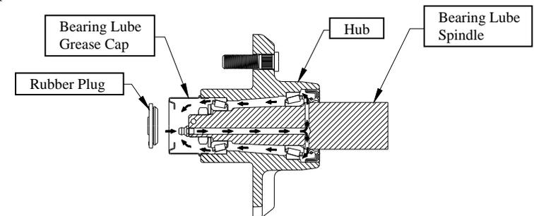
For units that are not equipped with the Sure Lube or Bearing Lube greasing system, the bearings must be packed with grease (by hand) prior to assembly, or at intervals as outlined in the maintenance schedule on page 28 of this manual.
