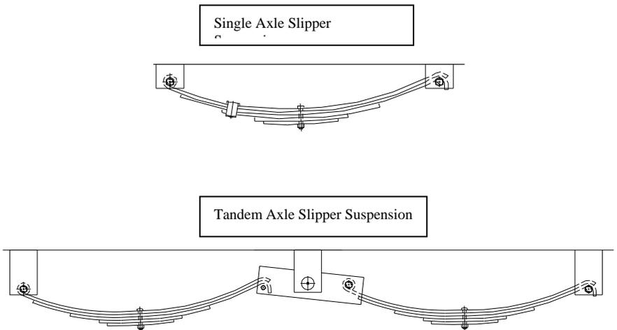
Slipper springs have an eye formed in one end only with the other end formed into a reverse curve. The attachment of these springs is as follows:
