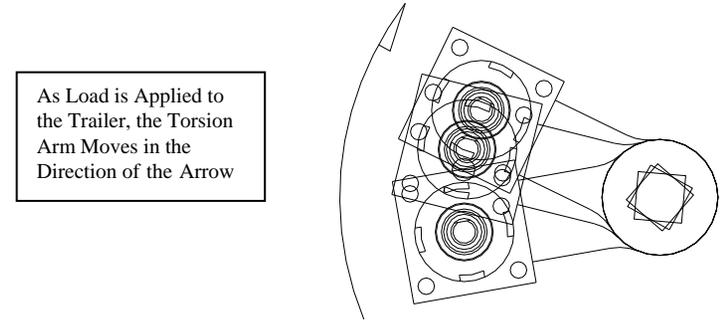
**How the Rubber Torsion Suspension System Works**
