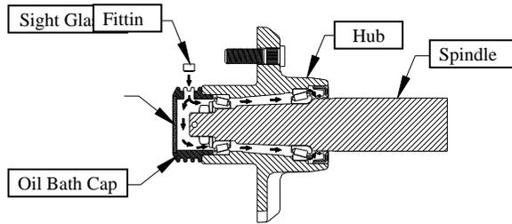
**2. Oil Bath Lubrication System – Plastic Cap**
