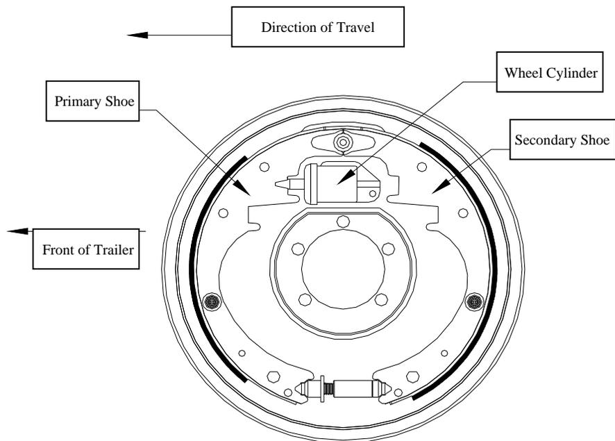
Make hard stops from 20 mph on a dry paved road free of sand and gravel. If the trailer brakes lock and slide, add more resistance to the circuit with
